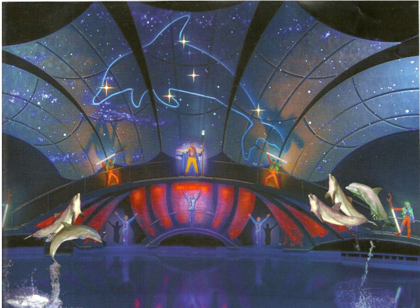
The five main projection surfaces, shaped like dolphin tails, were designed by Michael Hotopp. They are aluminum, painted with Screen-Gloss.
