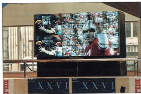
The Electrosonic PROCUBE 2 is a high brightness projection cube ideal for big image display. This unretouched photo of a 6x4 array shows its even illumination and suitability for high ambient light operation.
