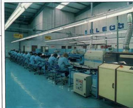
A corner of the Fairfax building. In the foreground a rolling production line, in the background SMT automatic assembly equipment.
