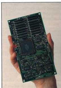
Celco AVIATOR uses parallel processing based on transputers.
