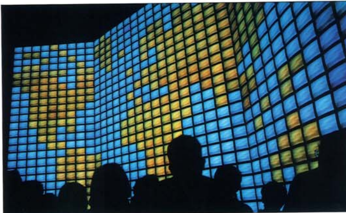
The "Global Village" videowall at EXPO 92, a 34x25 video wall. This photograph clearly shows the architect's "pixel" concept.
