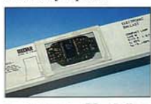
A cut-away LP ballast, showing the Neuron (R) chip.
