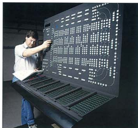
One of the mimic patch panels for TBS, under test at Hawley Mill.
