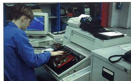
Automatic testing of dimmer circuit boards on a Marconi tester at Maidstone.
