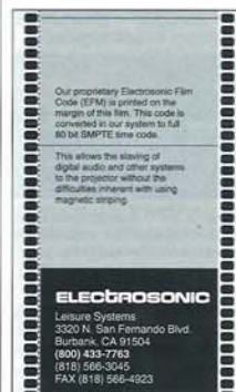
The EFM code is printed between the sprocket holes and the picture.
