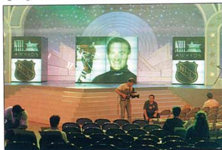
CBC used moving videowalls for the NHL Awards. Four 4x2, two 4x4, one 8x4, or two 4x2 and one 4x4 could all be shown.
