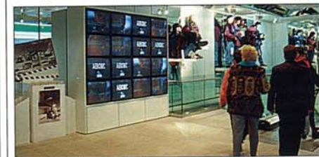
Electrosonic GmbH installed twin 4x4 PICBLOC-3 videowalls in the "Young Collection" C&A store in Cologne. Photo Wurdel & Schenck.
