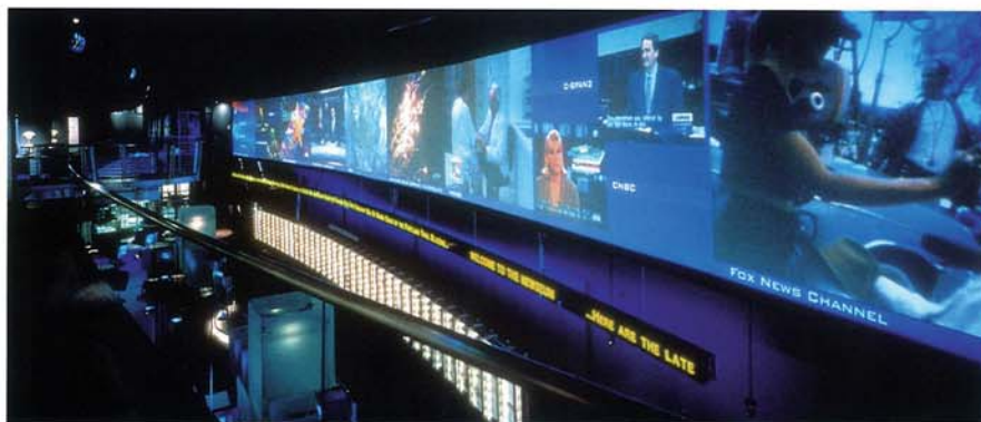
The News Wall at The Newseum is 126ft long. It can show up to 36 simultaneous images, each of which can be programmed to be any size and at any position in the display. Overall display resolution is 14400 x 1200.
