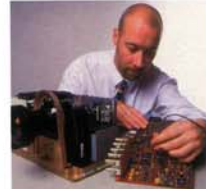
The projection "engine" used in Electrosonic's first DLP™ products. The Electrosonic interface is on the right.
