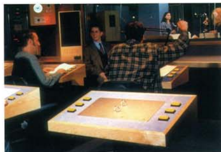
The popular interactive radio studio, where visitors record a radio drama. In the foreground are sound effects control panels driving Electrosonic ESTA digital sound stores.
