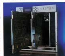
VECTOR's stylish housing is designed for EMC and for practical installation. Each unit can accommodate one system manager card, four 2-channel input cards, nine 4-channel output cards. All external connectors are at the back.
