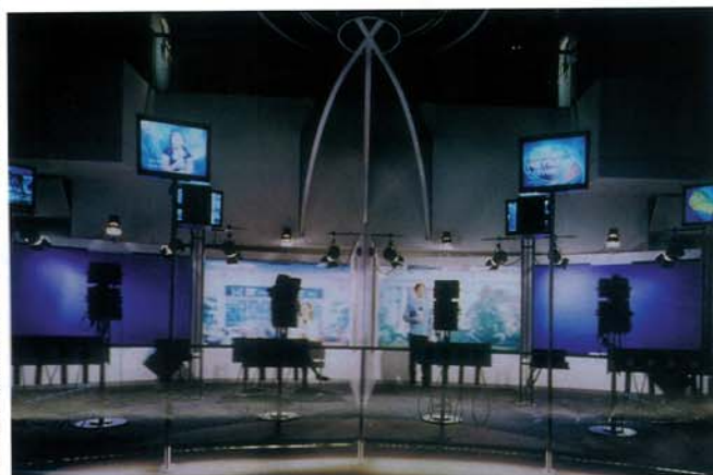
The four participatory exhibits at The Newseum. Two use blue screen, and two use scenic backdrops. All use professional prompting equipment and semi-professional cameras. Electrosonic engineered the interactive system, based on MPEG video compression and a computer local area network (LAN).
