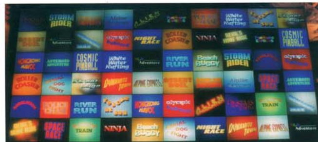
The 26ft (8m) wide 10x6 videowall on the Showscan booth at IAAPA '97. Here multiple "freezes" are used to show nearly 60 different images.
