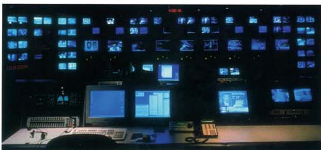
The production suite for the News Wall. There is a big monitor corresponding to each projector. Above each big monitor there are four small monitors corresponding to the four sources at present being used for that screen section. At the sides there are additional source monitors. In front there are two programming positions, allowing both on-line and off-line programming. In order to facilitate programming, there are two computer monitors for each programming computer.
